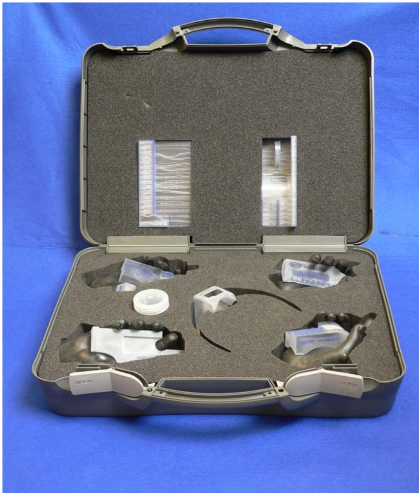
A complete 'CTIA hand kit hands, spacers, and alignment jigs, " all together ".
