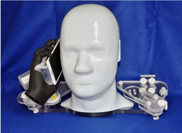
UWPDA hand mounted on IXBH-060 fixture for left and right device testing
